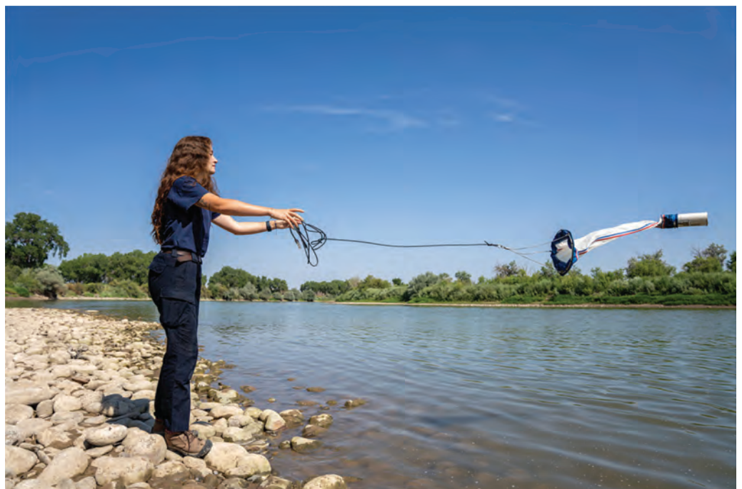
Colorado Parks and Wildlife invasive species specialist throws a plankton tow into the Colorado River to collect water samples for zebra mussel testing. (CPW/R. Gonzales)
