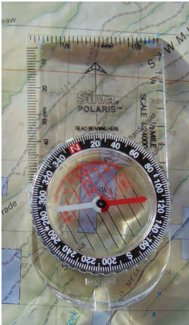
There is a difference between magnetic north and true north, and it is moving. (Submitted photo/Mark Rackay)
