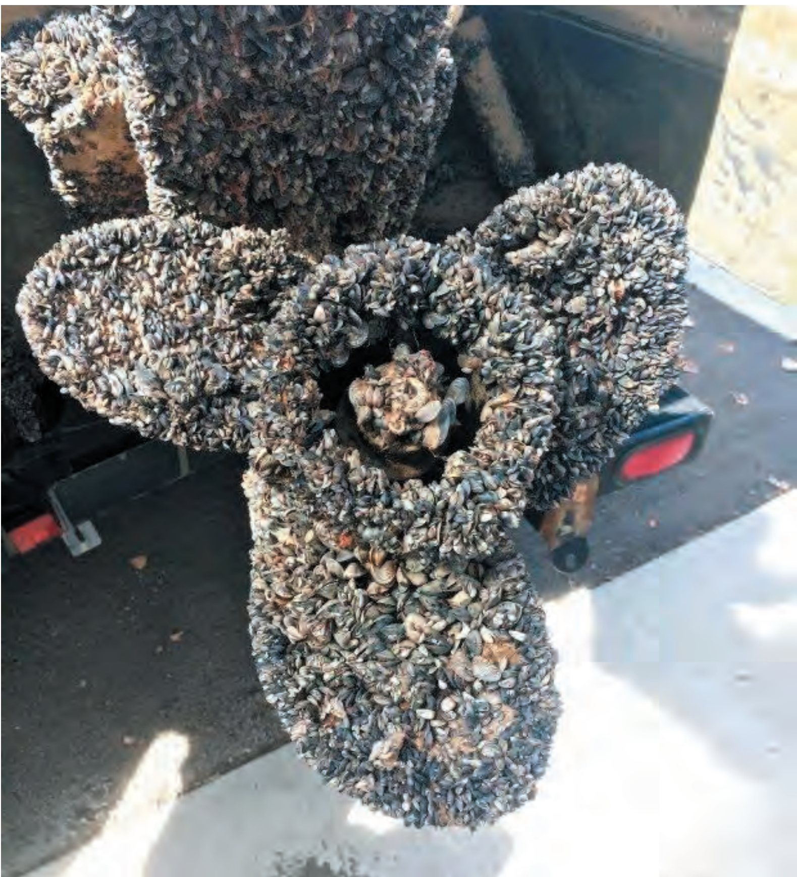
This is what zebra mussels do to the lower unit on an outdrive, similar to the saltwater barnacles. (Courtesy photo/Colorado Parks and Wildlife)
