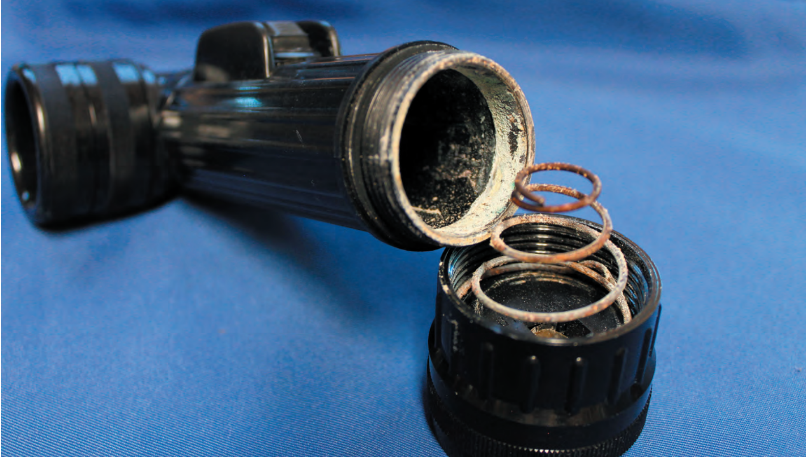
This ruined flashlight, caused by battery leakage, is just one of the reasons your outdoor equipment needs to be winterized. (Mark Rackay/Special to the Montrose Daily Press)
