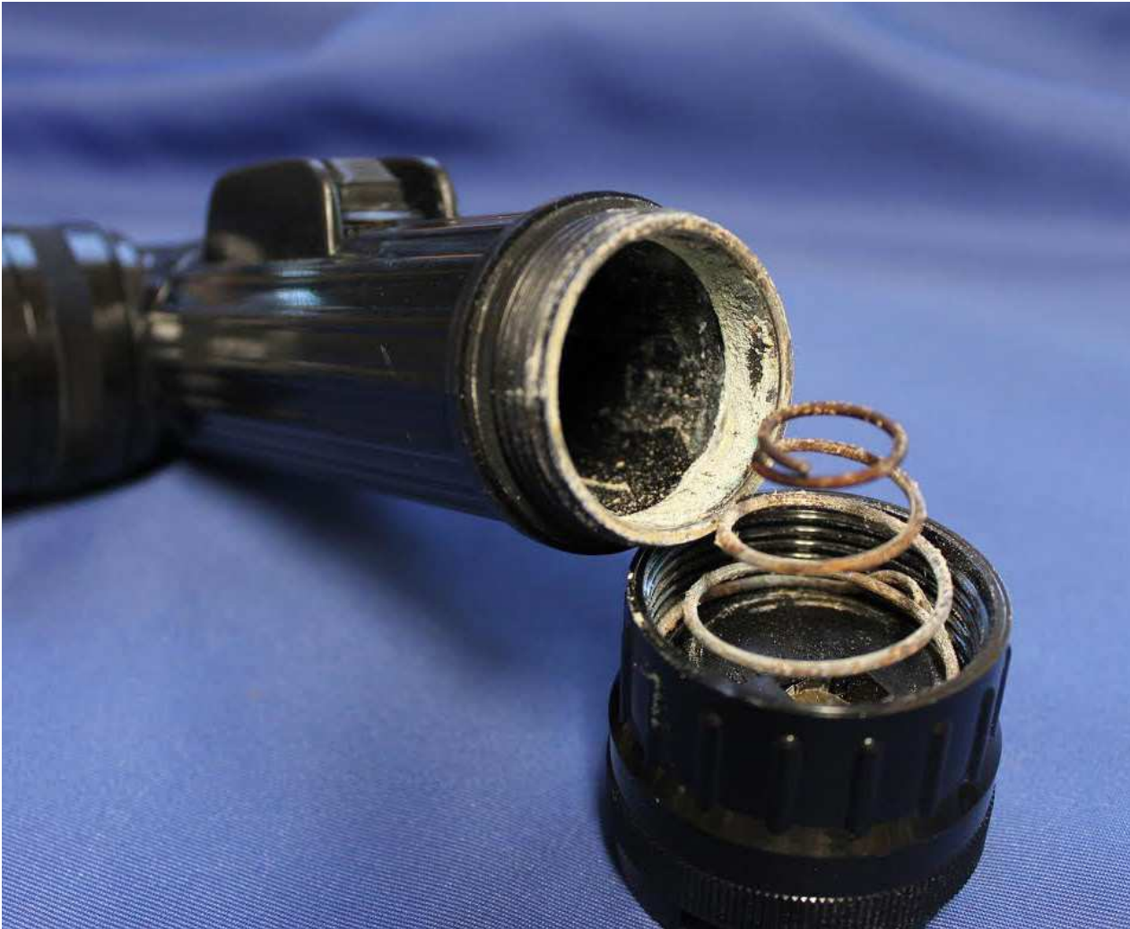
(Top) At first I thought Murphy had wrecked my flashlight, but soon realized it was my own fault. Battery neglect can ruin devices and equipment. (Submitted photo/Mark Rackay)
