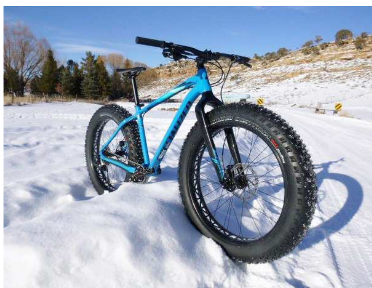
Typical fat bike. Note the large (5 inch wide) tires, wide rims and single chainring. The bike is geared low to help the rider climb better with the larger tires. (Courtesy photo)
